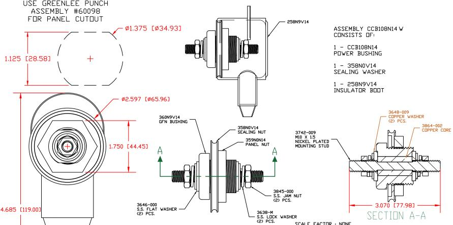
MAXIMUM FASTENER TORQUES: JAM NUTS: 212 IN-LBS [24.0 Nm] SEALING NUT: 120 IN-LBS [13.56 Nm]
